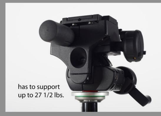
• I believe that there is small amount of movement inherent in the gear assembly. This allows it to move and to work in the first place, but this same slack allows a heavier camera to throw out camera to copy board alignment.
