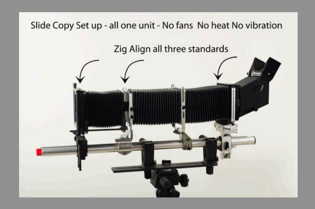
That old 8X10 rear standard may work in reverse to hold an 8X10 glass plate in place.
