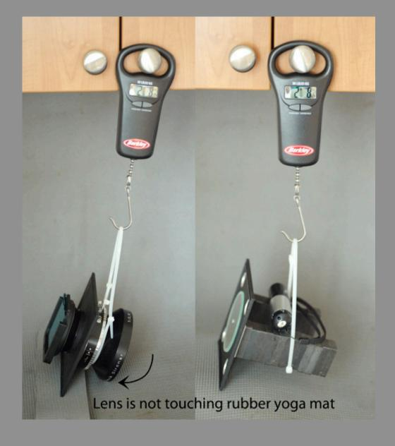
• A Digital Fish Scale to measure the downward force
